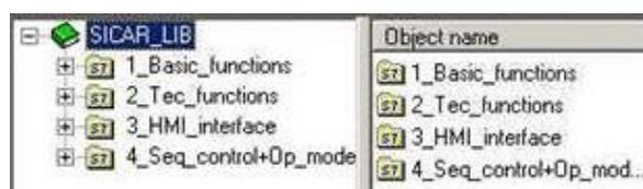
SICAR lib is a S7-library and consists of Basic\_functions, Tec-unit blocks, HMI\_interface and Sequence control incl. operation modes.
